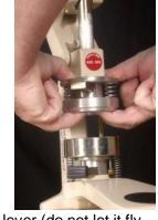
• Gently release the top lever (do not let it fly back to the vertical position). You will see that the white badge back remains in the bottom bit while the other components are in the top bit.
